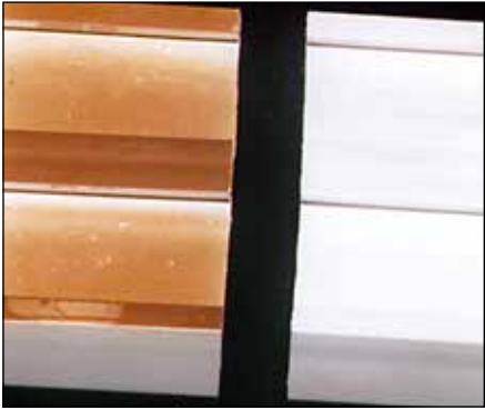
Figure 10: Discolouration of PVC-U under UV test - tested (left) and untested (right)
