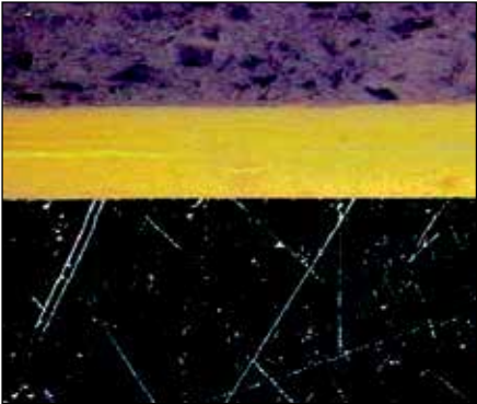
Figure 9: Aluminium cladding sample after the tests, with no sign of any corrosion @ magnification of 100
