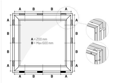
**Step 1.2** Fix the frame with wedges. The wedges must be positioned next to each fixing point on the window.
