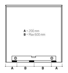
**Step 1.1** Place bearing pads at the bottom of the opening next to each fixing point on the window (A) and (B). If the window width is less than 1000 mm, bearing pads are only needed in position (A). Ensure they are level.
