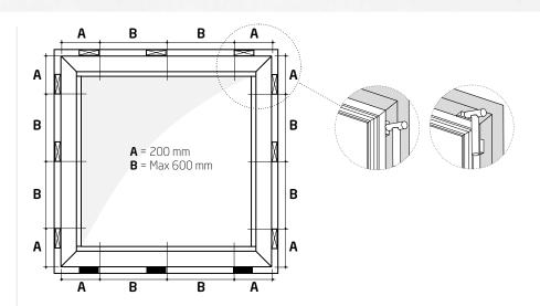
**Step 2.2** Fix the frame with wedges into the wall opening. Wedges must be positioned next to each fixing point on the window, beneath the frame.
