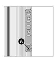
**Step 1.1** The bracket should be fitted in one line of the profile. Bracket "knobs" should be fitted in the grooves (A).
