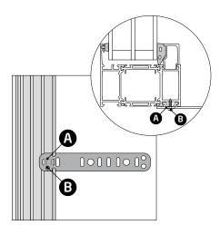
**Step 1.3** The bracket should be fastened to the frame with a screw (12165). One pc./bracket (B).
