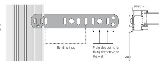
**Step 3.2** Fasten the window with the screws to the wall.
