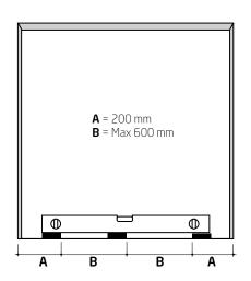
**Step 2.1** Place bearing pads at the bottom of the opening next to each fixing point on the window (A) and (B). If the window width is less than 1000 mm, bearing pads are only needed in position (A). Ensure they are level.
